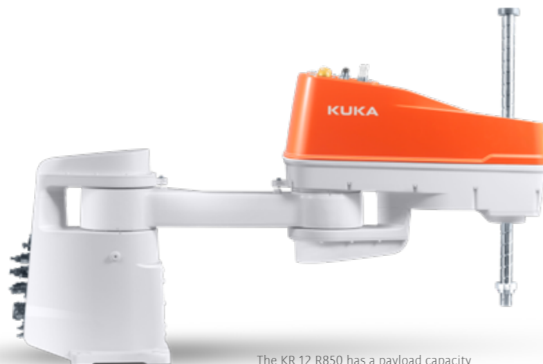
The KR 12 R850 has a payload capacity of 12 kilograms and a reach of 850 millimeters.
