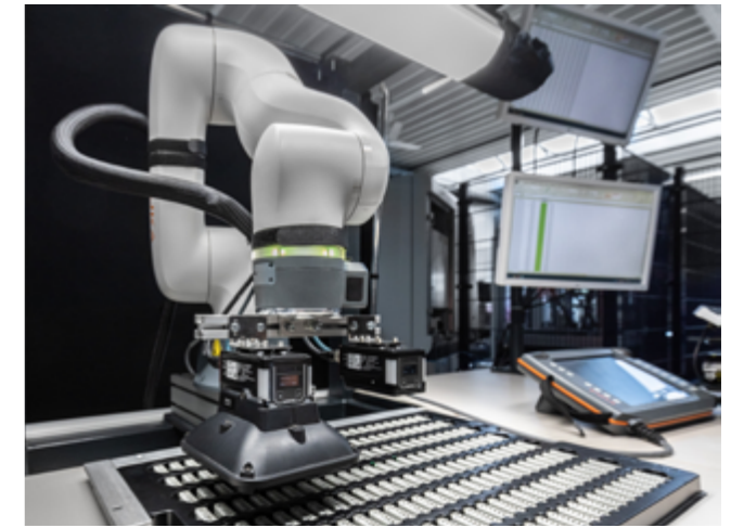
Equipped with cameras, an LBR iisy cobot in conjunction with the iiQKA.OS operating system, checks quality in the plastics industry.
