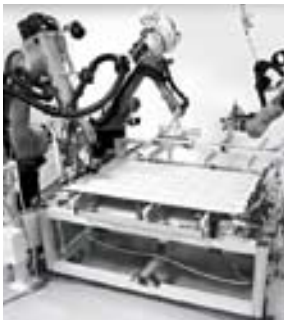
Solar module cross connect station.
