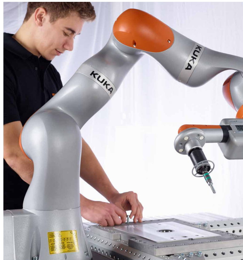
The sensitive LBR iiwa lightweight robot supports humans through direct collaboration.
