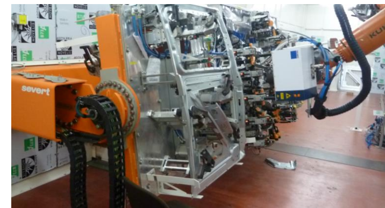
Remote Welding of doors
