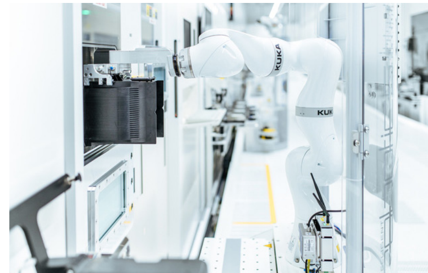
In the cleanroom, humans and machines work "hand in hand" in many ways. A mobile cobot can be an alternative to costly and technically complex Overhead Transport Systems (OHT)
