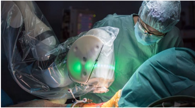
The laser head – held by a KUKA LBR Med – enables bone surgery to be performed with unprecedented precision. (© AO Davos/AOT)
