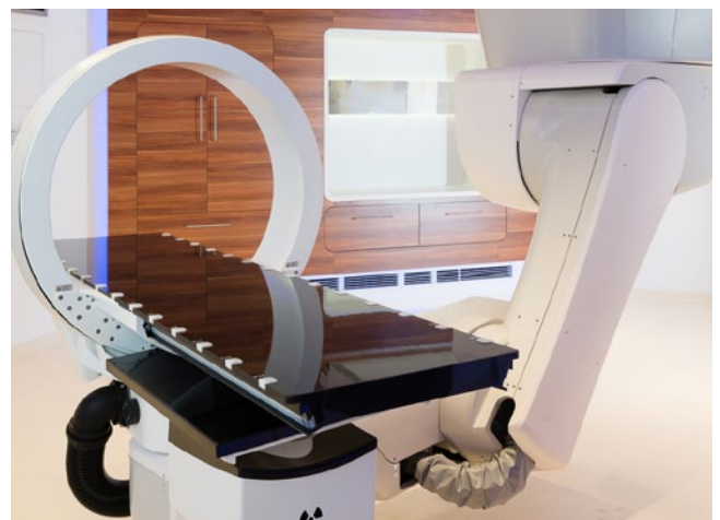
BEC uses KUKA robots for precise positioning of the patient during particle-based radiation therapy (© Thomas Kästenbauer)
