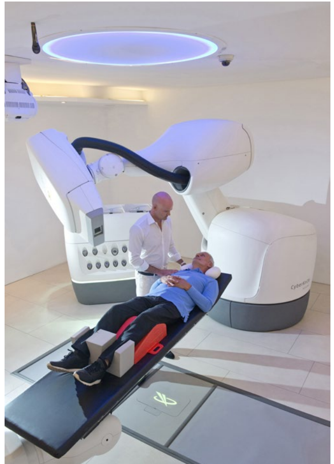
The patient lies freely positioned on the robotically controlled treatment table while the CyberKnife treats the tumor.
