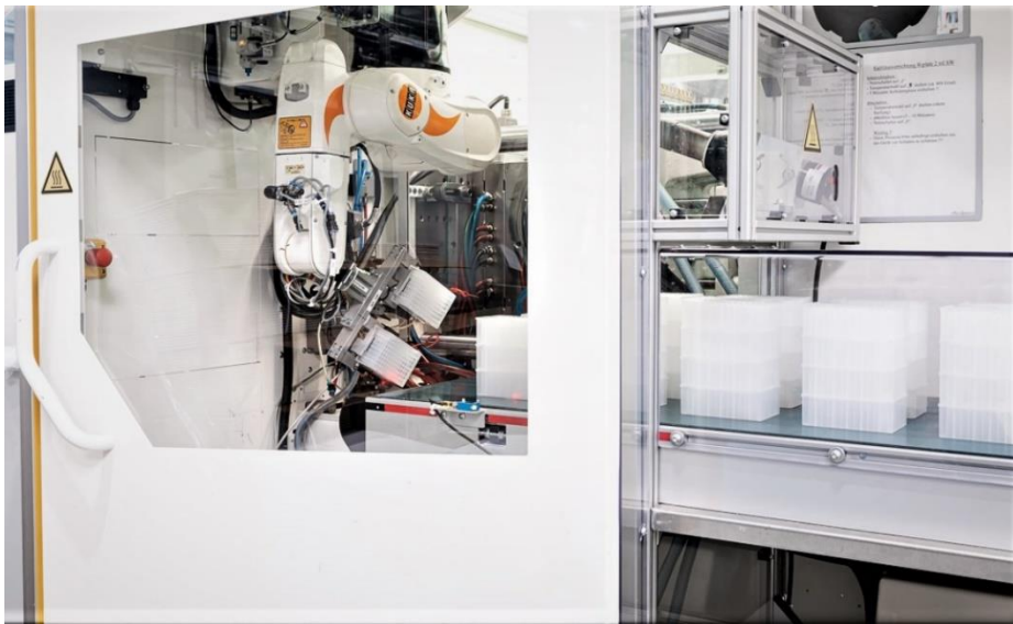
A fixed component for several years now: KUKA robots in an injection molding system that produces medical material for laboratories from plastic. © Ritter GmbH
