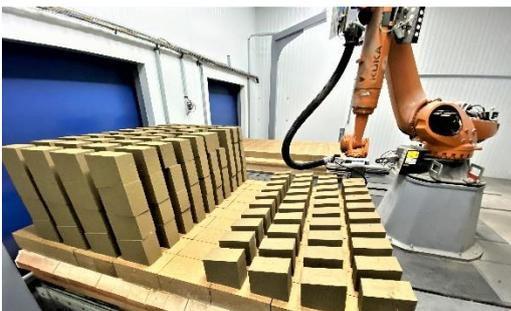
*The camera helps the robot to detect the exact position of the kiln bricks. © Kautenburger GmbH*
