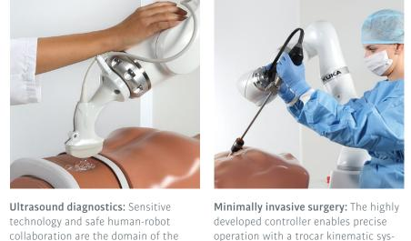
collaboration are the domain of the LBR Med. Thanks to the integrated Open-source libraries facilitate the fast sensors, it can react to its surroundings to use the application automatically, both interactively with the physician and via telemanipulation.
