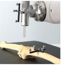
Orthopedic surgery: Thanks to its stable design and construction, as well as its high stiffness, the LBR Med is particularly suitable for bone surgery. development of prototypes and the integration of navigation cameras.
