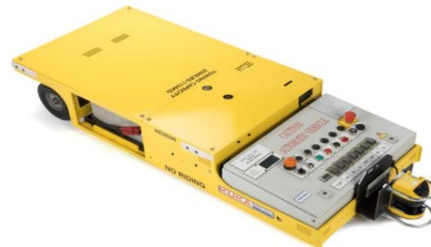
**KUKA Mor-Tech** automated guide carts are a low cost, easy to operate, easy to maintain way to optimize processes across your manufacturing needs. Material handling to assembly applications, each AGC provides an unbeatable combination of safety, performance and reliability.
