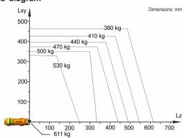
The KR 500 R2830 is designed for a rated payload of 500 kg in order to optimize the dynamic performance of the robot. The maximum payload of 611 kg applies only if the position of the center of mass is 0 mm and a supplementary load optimized for the load case is mounted. The specific load case must be verified using KUKA.Load or KUKA Compose. For further consultation, please contact KUKA Support.
