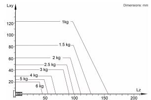
The KR 3 D1200 HM is designed for a rated payload of 3 kg in order to optimize the dynamic performance of the robot. With reduced load center distances and favorable supplementary loads, a maximum payload of up to 6 kg can be mounted. The specific KUKA Load case must be verified using KUKA. For further consultation, please contact KUKA Service.
