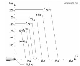
The KR 10 R900-2 is designed for a rated payload of 5 kg in order to optimize the dynamic performance of the robot. The maximum payload of 11.3 kg applies only if the position of the center of mass is 0 mm and a supplementary load optimized for the load case is mounted. The specific load case must be verified using KUKA.Load or KUKA Compose. For further consultation, please contact KUKA Support.
