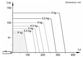
The KR 6 R900 WP is designed for a rated payload of 3 kg in order to optimize the dynamic performance of the robot. The maximum payload of 6 kg applies only if the position of the center of mass is 0 mm and a supplementary load optimized for the load case is mounted. The specific load case must be verified using KUKA.Load or KUKA Compose. For further consultation, please contact KUKA Support.
