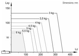
The KR 6 R700 CR is designed for a rated payload of 3 kg in order to optimize the dynamic performance of the robot. The maximum payload of 6 kg applies only if the position of the center of mass is 0 mm and a supplementary load optimized for the load case is mounted. The specific load case must be verified using KUKA.Load or KUKA Compose. For further consultation, please contact KUKA Support.
