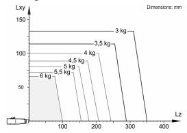
The KR 6 R900 CR is designed for a rated payload of 3 kg in order to optimize the dynamic performance of the robot. The maximum payload of 6 kg applies only if the position of the center of mass is 0 mm and a supplementary load optimized for the load case is mounted. The specific load case must be verified using KUKA.Load or KUKA Compose. For further consultation, please contact KUKA Support.
