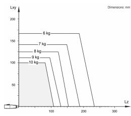
The KR 10 R900 CR is designed for a rated payload of 5 kg in order to optimize the dynamic performance of the robot. The maximum payload of 10 kg applies only if the position of the center of mass is 0 mm and a supplementary load optimized for the load case is mounted. The specific load case must be verified using KUKA.Load or KUKA Compose. For further consultation, please contact KUKA Support.
