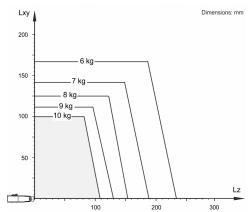
The KR 10 R1100 CR is designed for a rated payload of 5 kg in order to optimize the dynamic performance of the robot. The maximum payload of 10 kg applies only if the position of the center of mass is 0 mm and a supplementary load optimized for the load case is mounted. The specific load case must be verified using KUKA.Load or KUKA Compose. For further consultation, please contact KUKA Support.
