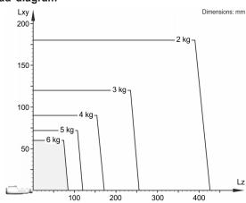
The KR 6 R700 HM-SC is designed for a rated payload of 3 kg in order to optimize the dynamic performance of the robot. The maximum payload of 6 kg applies only if the position of the center of mass is 0 mm and a supplementary load optimized for the load case is mounted. The specific load case must be verified using KUKA.Load or KUKA Compose. For further consultation, please contact KUKA Support.
