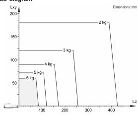
The KR 6 R900 HM-SC is designed for a rated payload of 3 kg in order to optimize the dynamic performance of the robot. The maximum payload of 6 kg applies only if the position of the center of mass is 0 mm and a supplementary load optimized for the load case is mounted. The specific load case must be verified using KUKA.Load or KUKA Compose. For further consultation, please contact KUKA Support.
