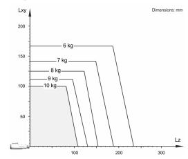
The KR 10 R900 HM-SC is designed for a rated payload of 5 kg in order to optimize the dynamic performance of the robot. The maximum payload of 10 kg applies only if the position of the center of mass is 0 mm and a supplementary load optimized for the load case is mounted. The specific load case must be verified using KUKA.Load or KUKA Compose. For further consultation, please contact KUKA Support.
