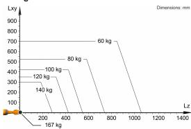
The KR 120 R2700-2 is designed for a rated payload of 120 kg in order to optimize the dynamic performance of the robot. The maximum payload of 167 kg applies only if the position of the center of mass is 0 mm and a supplementary load optimized for the load case is mounted. The specific load case must be verified using KUKA.Load or KUKA Compose. For further consultation, please contact KUKA Support.
