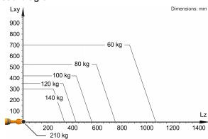
The KR 120 R3100-2 is designed for a rated payload of 120 kg in order to optimize the dynamic performance of the robot. The maximum payload of 210 kg applies only if the position of the center of mass is 0 mm and a supplementary load optimized for the load case is mounted. The specific load case must be verified using KUKA.Load or KUKA Compose. For further consultation, please contact KUKA Support.
