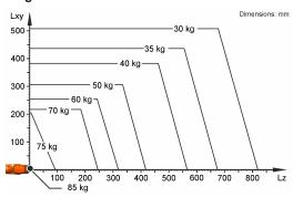
The KR 70 R2100 is designed for a rated payload of 70 kg in order to optimize the dynamic performance of the robot. With reduced load center distances and favorable supplementary loads, a maximum payload of up to 85 kg can be mounted. The specific KUKA Load case must be verified using KUKA. For further consultation, please contact KUKA Service.
