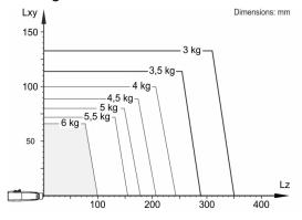
The KR 6 R900 EX is designed for a rated payload of 3 kg in order to optimize the dynamic performance of the robot. The maximum payload of 6 kg applies only if the position of the center of mass is 0 mm and a supplementary load optimized for the load case is mounted. The specific load case must be verified using KUKA.Load or KUKA Compose. For further consultation, please contact KUKA Support.
