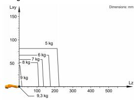
The KR 8 R2100-2 arc HW is designed for a rated payload of 8 kg in order to optimize the dynamic performance of the robot. The maximum payload of 9.3 kg applies only if the position of the center of mass is 0 mm and a supplementary load optimized for the load case is mounted. The specific load case must be verified using KUKA.Load or KUKA Compose. For further consultation, please contact KUKA Support.
