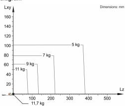
The LBR iisy 11 R1300 is designed for a rated payload of 11 kg in order to optimize the dynamic performance of the robot. The maximum payload of 11.72 kg only applies if the position of the center of mass is 0 mm. The specific load case must be verified using KUKA.Load or KUKA Compose. For further consultation, please contact KUKA Support.
