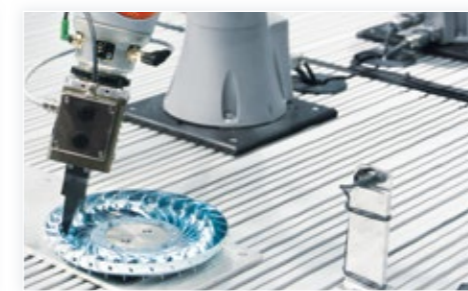
PRECISE ASSEMBLY: In the assembly of torque converter transmissions, the LBR iiwa positions delicate converter blades with uncompromising precision, without the need for complex tools, external sensors or actuators.
