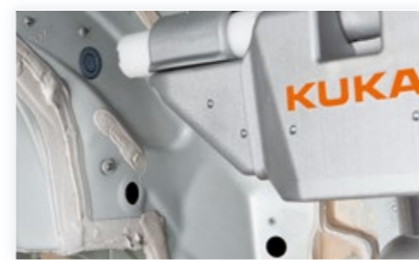
EXACTLY THE RIGHT PART: Even if assembly parts are not precisely positioned in the magazine, the LBR iiwa can detect their position and assemble them perfectly.
