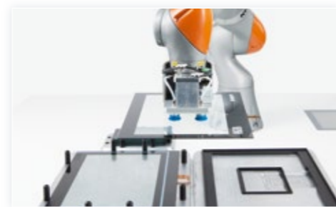
PERFECT POSITIONING: With the LBR iiwa, assembly parts can be aligned and joined precisely without the need for additional sensors. One example is display glass assembly in the electronics sector.
