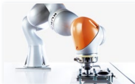
INSERTING PLUGS: In the assembly of flexible automotive parts, the LBR iiwa performs non-ergonomic and monotonous tasks with the utmost reliability.
