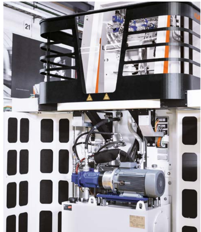
Integrated hydraulic cabinet with generously dimensioned maintenance doors
