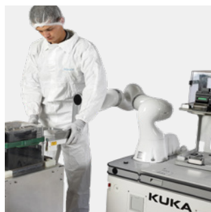
The sensitive LBR iiwa 14 R820 CR enables collaboration in the same workspace without safety fencing
