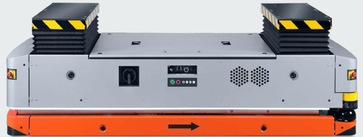
**Unrestricted and precise maneuvering** Thanks to KUKA omniMove drive technology, the KMP 1500 can move in any direction from a standing position. The sophisticated wheel technology allows for precise positioning with an accuracy of ±5 millimeters even in tight spaces. This results in space-saving and highly precise automation solutions for logistics.
