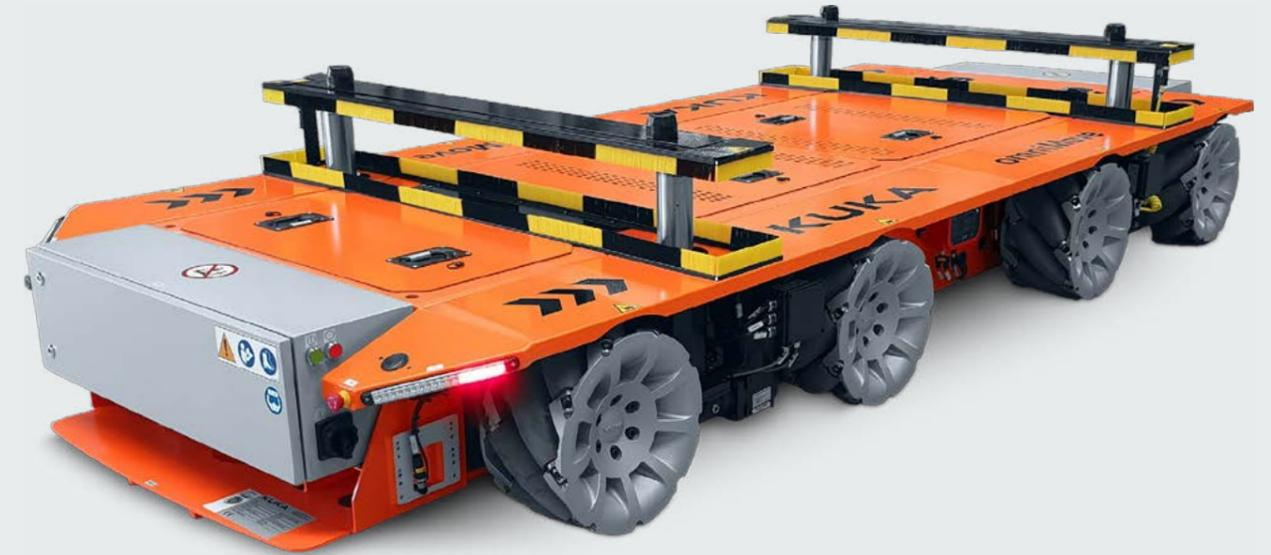
**Powerful.** Depending on the vehicle variant, the KUKA omniMove can safely and conveniently move even the heaviest components in XXL format. It has a payload capacity of up to 90 tonnes and – in the maximum version – reaches a length up to 30 meters.
