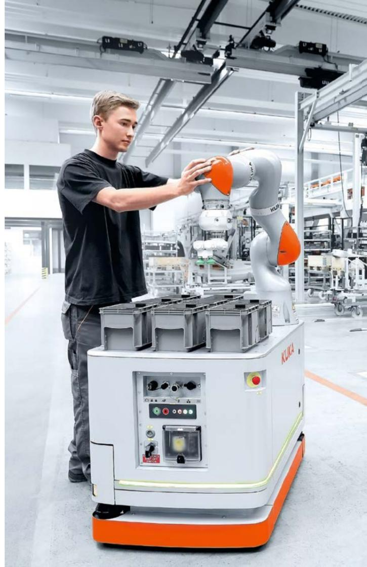
**Combinable.** Design your individual turnkey system solution. The modular KMR iiwa system offers numerous combinations of robot technology, mobile platforms and industrial components.
