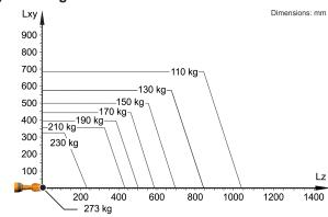
The KR 210 R3300-2 K is designed for a rated payload of 210 kg in order to optimize the dynamic performance of the robot. The maximum payload of 273 kg applies only if the position of the center of mass is 0 mm and a supplementary load optimized for the load case is mounted. The specific load case must be verified using KUKA.Load or KUKA Compose. For further consultation, please contact KUKA Support.
