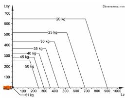
The KR 50 R2500 is designed for a rated payload of 50 kg in order to optimize the dynamic performance of the robot. With reduced load center distances and favorable supplementary loads, a maximum payload of up to 61 kg can be mounted. The specific KUKA Load case must be verified using KUKA. For further consultation, please contact KUKA Service.
