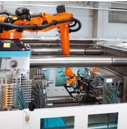
On the machine: KUKA QUANTEC shelf-mounted robots for efficient loading, unloading and finishing
