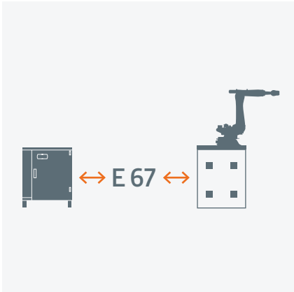
EUROMAP E67 interface It regulates the safe signal exchange on the basis of a standardized dialog between the machine and the robot.
