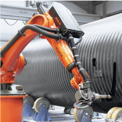
In the system: precise milling of overdimensional plastic pipes
