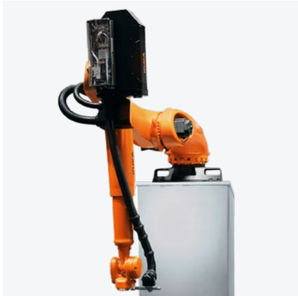
KR QUANTEC K series KUKA shelf-mounted robots are designed for an especially large downward reach. They optimally access the workspace from above.
