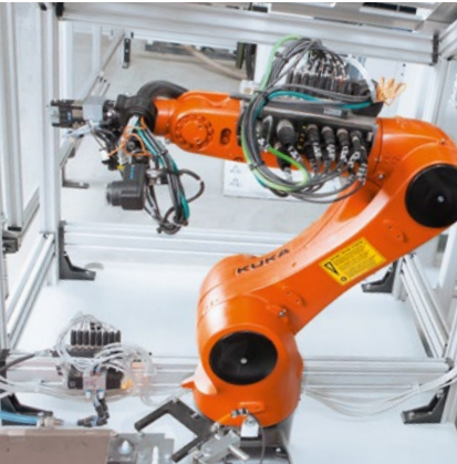
In the system: A space-saving KR AGILUS carries out positioning tasks and accesses the assembly fixture from underneath.
