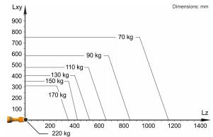
The KR 150 R3100-2 is designed for a rated payload of 150 kg in order to optimize the dynamic performance of the robot. The maximum payload of 220 kg applies only if the position of the center of mass is 0 mm and a supplementary load optimized for the load case is mounted. The specific load case must be verified using KUKA.Load or KUKA Compose. For further consultation, please contact KUKA Support.
