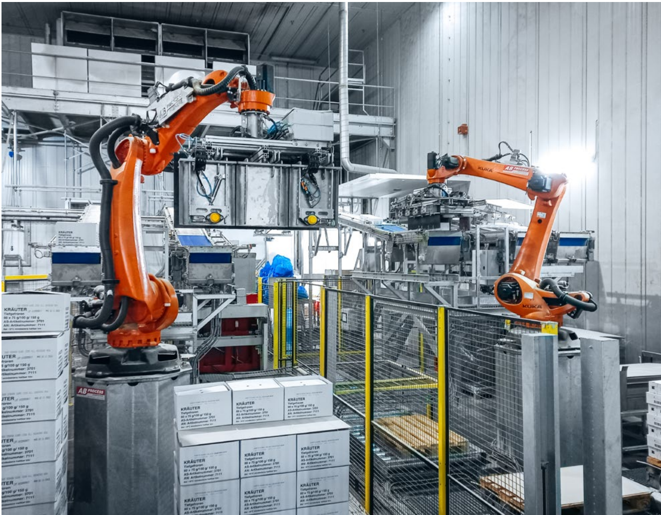
Under Arctic conditions at -25 °C, two KR QUANTEC PA Arctic robots palletize frozen aromatic herbs.
