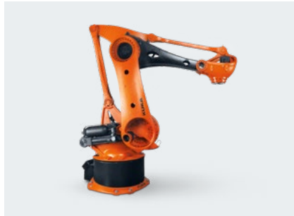
KR 700 PA The low weight and powerful motors and gear units make it a real high-speed champion.
