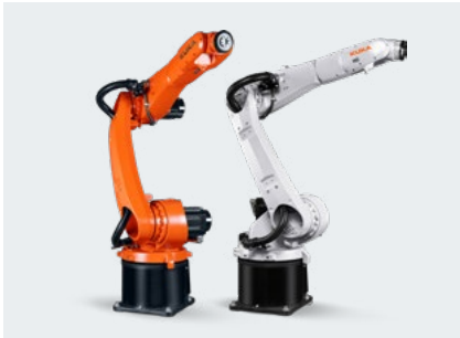
KR CYBERTECH nano (HO) The process robots are perfectly tailored to handling small food and packaging items. The diversity of variants enables optimized investment and energy costs.
