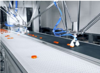
KUKA.PickControl The software automatically adapts the robot to the motion of an assembly line / conveyor belt. In this way, parts on the conveyor can be processed and placed on top of one another.
