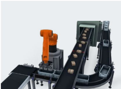
KUKA.ConveyorTech The technology package with integrated image processing enables automated picking & packing of unsorted parts – for example, fruit on multiple assembly lines / conveyor belts.
