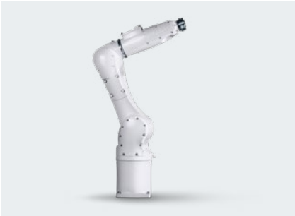
KR AGILUS HM Corrosion-resistant surfaces, food-compatible lubricants and stainless steel parts ensure the highest level of hygiene. It is thus perfectly suited for sterile environments.
