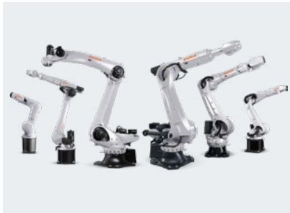
The KUKA HO robot portfolio Food-compatible H1 lubricants in all axes: the “Hygienic Oil” (HO) variants meet the high requirements of the foodstuffs industry – for hygienic handling with no compromises. KUKA offers outstanding efficiency and the world’s broadest portfolio in this area.
