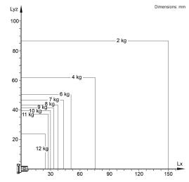
The KR 12 R850 Z340 CR is designed for a rated payload of 6 kg in order to optimize the dynamic performance of the manipulator. With the reduced load center distances, higher loads up to the maximum payload may be used. The specific load case must be verified using KUKA.Load. For further consultation, please contact KUKA Support.
