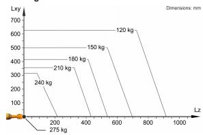
The KR 210 R2700-2 F is designed for a rated payload of 210 kg in order to optimize the dynamic performance of the robot. The maximum payload of 275 kg applies only if the position of the center of mass is 0 mm and a supplementary load optimized for the load case is mounted. The specific load case must be verified using KUKA.Load or KUKA Compose. For further consultation, please contact KUKA Support.
