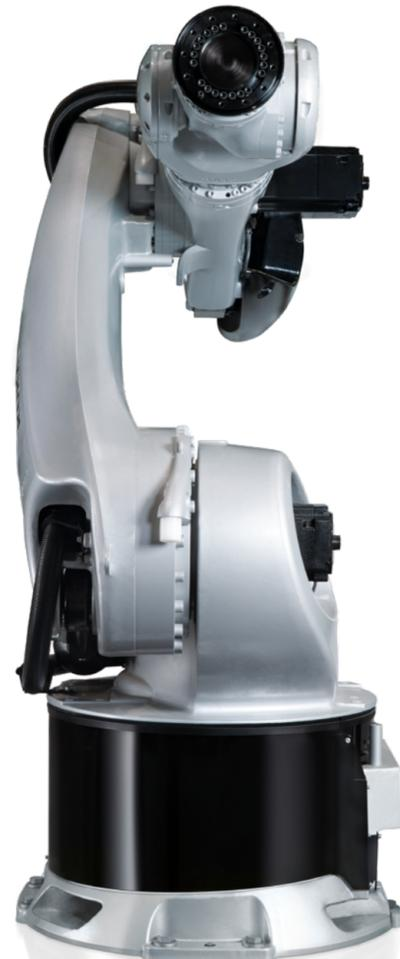
**One robot, endless application possibilities.** Thanks to its six freely programmable axes, the KR 600 R2830 passenger simulates each motion sequence with absolute precision and a highly dynamic performance. Up to three people can experience the hair-raising ride at the same time thanks to the overall payload capacity of 600 kg.
