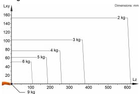
The KR 6 R1440-2 arc HW E is designed for a rated payload of 6 kg in order to optimize the dynamic performance of the robot. With reduced load center distances and favorable supplementary loads, a maximum payload of up to 9 kg can be mounted. The specific KUKA Load case must be verified using KUKA. For further consultation, please contact KUKA Service.
