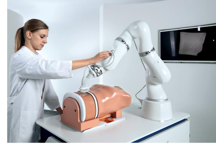
Ultrasound diagnostics: Sensitive technology and safe human-robot collaboration are the domain of the LBR Med. Thanks to the integrated sensors, it can react to its surroundings both interactively with the physician and via telemanipulation.
