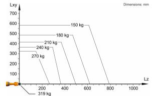
The KR 240 R2900-2 F is designed for a rated payload of 240 kg in order to optimize the dynamic performance of the robot. The maximum payload of 319 kg applies only if the position of the center of mass is 0 mm and a supplementary load optimized for the load case is mounted. The specific load case must be verified using KUKA.Load or KUKA Compose. For further consultation, please contact KUKA Support.
