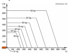
The KR 50 R2500 F is designed for a rated payload of 50 kg in order to optimize the dynamic performance of the robot. With reduced load center distances and favorable supplementary loads, a maximum payload of up to 61 kg can be mounted. The specific KUKA Load case must be verified using KUKA. For further consultation, please contact KUKA Service.
