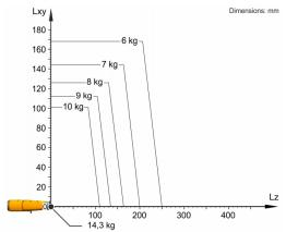
The KR 10 R1440-2 is designed for a rated payload of 10 kg in order to optimize the dynamic performance of the robot. The maximum payload of 14.3 kg applies only if the position of the center of mass is 0 mm and a supplementary load optimized for the load case is mounted. The specific load case must be verified using KUKA.Load or KUKA Compose. For further consultation, please contact KUKA Support.
