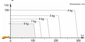
The KR 8 R1420 arc HW is designed for a rated payload of 8 kg in order to optimize the dynamic performance of the robot. With reduced load center distances, higher loads up to the maximum payload may be used. The specific load case must be verified using KUKA.Load. For further consultation, please contact KUKA Support.
