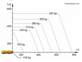
The KR 340 R3330 F is designed for a rated payload of 340 kg in order to optimize the dynamic performance of the robot. The maximum payload of 418 kg applies only if the position of the center of mass is 0 mm and a supplementary load optimized for the load case is mounted. The specific load case must be verified using KUKA.Load or KUKA Compose. For further consultation, please contact KUKA Support.
