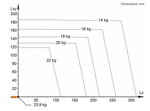
The KR 20 R1820-2 E is designed for a rated payload of 20 kg in order to optimize the dynamic performance of the robot. With reduced load center distances and favorable supplementary loads, a maximum payload of up to 23.9 kg can be mounted. The specific KUKA Load case must be verified using KUKA. For further consultation, please contact KUKA Service.
