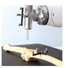
**Orthopedic surgery:** Thanks to its stable design and construction, as well technology and safe human-robot as its high stiffness, the LBR Med is suitable for bone surgery. Open-source LBR Med. Thanks to the integrated libraries facilitate the fast development sensors, it can react to its surroundings to use the application automatically, of prototypes and the integration of navigation cameras.
