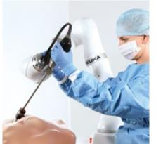
Minimally invasive surgery: The highly developed controller enables precise operation with a trocar kinematic system. The user can freely select whether interactively or via a telemanipulator.
