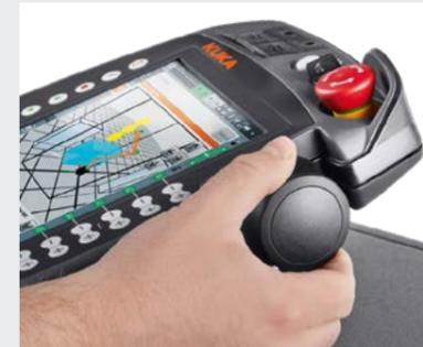
**Simple robot jogging with the ergonomic 6D mouse.** It offers intuitive jogging and reorientation of the robot in three or six degrees of freedom.
