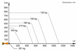
The KR 210 R3100-2 F is designed for a rated payload of 210 kg in order to optimize the dynamic performance of the robot. The maximum payload of 281 kg applies only if the position of the center of mass is 0 mm and a supplementary load optimized for the load case is mounted. The specific load case must be verified using KUKA.Load or KUKA Compose. For further consultation, please contact KUKA Support.
